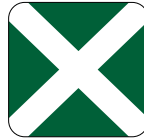
EMERGENCY MEDIAN CROSSING
