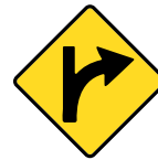
SIDE ROAD INTERSECTION ON A CURVE (R)
