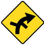
SUCCESSIVE SIDE ROAD INTERSECTIONS CURVE (R)
